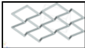
Fig. 3. Figure 3. OLEX depiction of the (6,3)-honeycomb topology, shown projected against the unit cell.
